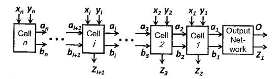
Cell i calculates  $a_i$ ,  $b_i$ , and  $Z_{i+1}$  by the following equations for  $i = 1 \sim n - 1$ .
