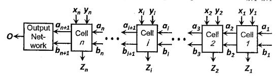
Cell i calculates  $a_{i+1}$ ,  $b_{i+1}$ , and  $Z_i$  by the following equations for  $i=1 \sim n$ .  $a_{i+1}=x_i'y_i'b_i+x_ib_i'+x_ia_i$  and  $b_{i+1}=x_i'a_i+y_ib_i'+x_iy_i'b_i$   $Z_i=y_i'+x_i'y_ia_ib_i'+x_ib_i$
