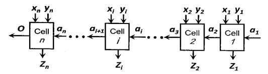
Cell i calculates  $a_{i+1}$  and  $Z_i$  by the following equations for  $i = 1 \sim n$ .
