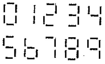
Figure 1. (a) Decimal digits displayed on 7-segment display elements.
