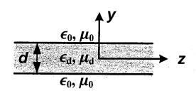
9. (10%) A waveguide consists of an infinite dielectric slab with permittivity  $\epsilon_d = 11.7\epsilon_0$ , permeability  $\mu_d = \mu_0$ , and thickness of 1 mm. It is sitting on a perfect conductor. What are the propagating modes and what are their cutoff frequencies of the lowest-order mode?
